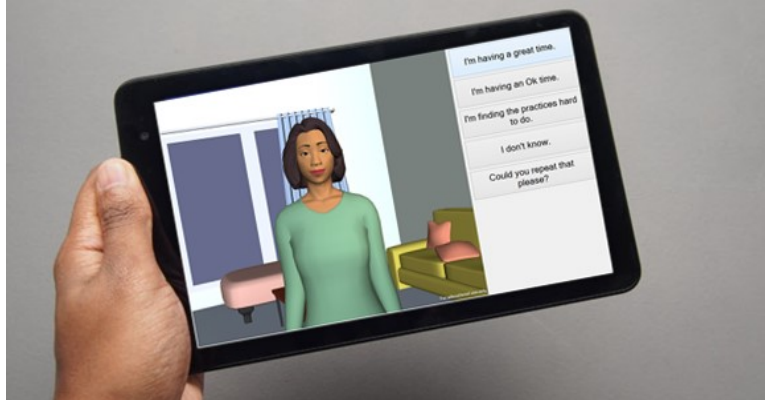
Fig. 1. Touch Screen Tablet Computer with Conversational Agent custom hierarchical transition network-based scripting language. User input is obtained via multiple choice selection of utterances on the touch screen [27].
